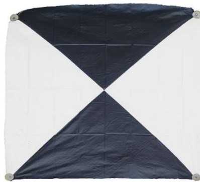
Fig. 6: A sample GCP (As placed on a concrete 18 X 18cm concrete beacon)
